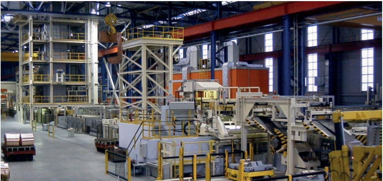
Strip width 600 – 1,250 mm | Strip thickness 0.3 – 6 mm | High temperature furnace up to 1,000 °C
